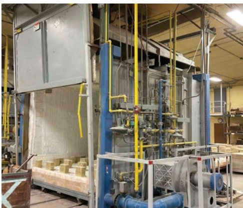
77 American gas fired car bottom shuttle kiln, 108"x160", (6) 104x52" cars, fiber lined, (6) bottom & (4) top NA Tempest burners, NA 15 hp. 1400 cfm combustion blower, SS0, power doors, in-floor rails, chain type car mover, Yokogawa 3-zone temperature control
