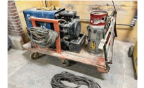
259 Miller Bobcat 225G portable welder/8,000 watt generator, s/nKG251837, Onan 16 hp. LP gas eng.,cart
