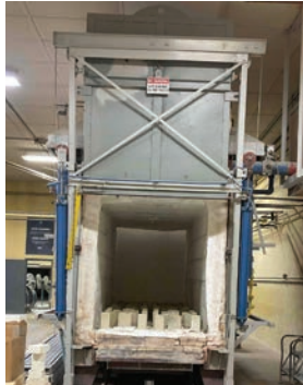
102 Ohio gas fired car bottom shuttle kiln, 80"x164", (2) 53x176" cars, above floor rail & chain car mover, (6) bottom & chain car mover, (3) top NA4422 burners, SSO, pneumatically powered doors. Note: If outside valving is removed furnace can be moved through the doors. Seller not responsible for moving
