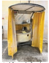
385 Central Ceramic Services spray glazing touch up unit, 36" dia. screen table, poly tub, De Vilbiss gun, Dayton 16" 1/2 hp. exhaust fan, curtain
