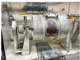
307 Abbe 36" dia. x 48" steel drum ball mill, 5 hp. electric drive, 230 volt
