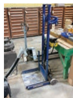
27 T & S 500 pound platform lift, Model# LLPH-500-FW, w/ Enerpac Hyd. Pump
