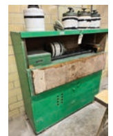
319 Ohio kilns double deck jar Mill with 4- 8" x 8" Porcelain Jars
