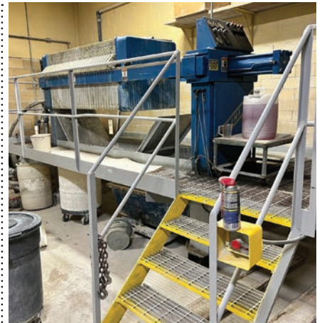
217 WI hydraulic 15 cu. ft. filter press, model 800G32-29-15DYLs, s/n F05456,(1995),(30)31.5x31.5" plates, steel platform, diaphragm pump, (2) rolling steel sludge tanks
