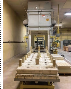
105 Denver I gas-fired car bottom shuttle kiln, model M-464, s/n 135,2500 deg F max temp, 94"x171", (4) 53x86" cars, above floor rail; chain car mover, power doors, Yokogawa 4-zone temperature control Note: If outside valving is removed furnace can be moved through the doors. Seller not responsible for moving
