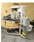
387 Malkin type 310 waterfall glazing machine's/n 9908/M1839/117/310, 4' dia. screen table, poly tub, Gusher 1 hp.pump
