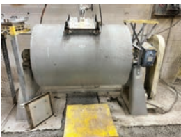
306 Abbe 36" dia. x 48" steel drum ball mill, model 5APM, SN A38788 Dorris Gear Reducer, motor drive
