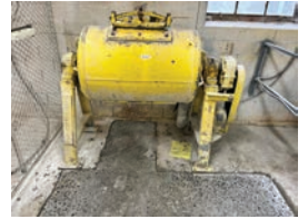
305 Patterson 24" dia.x 36" steel drum ball mill, electric drive
