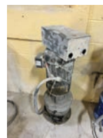
233 Sumitomo High speed Gear-box 10hp 3-phase, 230/460 volt
