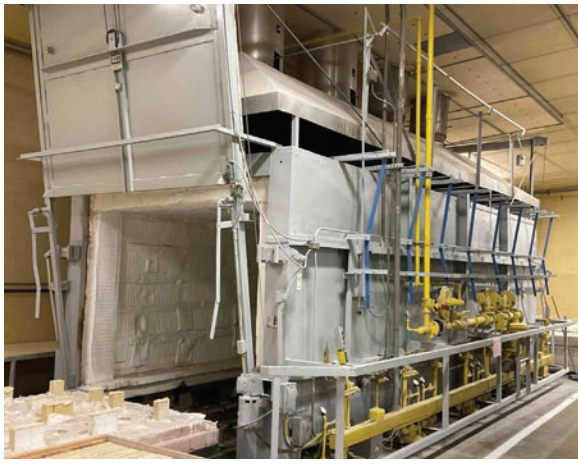
87 Denver II gas-fired car bottom shuttle kiln, model L67518, s/n 142, (1970), 2300 deg F max temp, 118"x315", (8)77x86" cars, above floor rail & chain car mover, West 2072 temperature control
