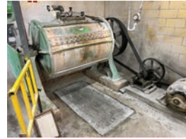
304 Patterson 30" dia.x 42" steel drum ball mill, electric drive
