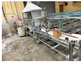
362 Custom built 4-nozzle spray glazing machine, rubber band conveyor, Gusher pump
