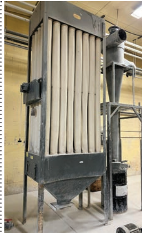
219 Dustkop 40-bag dust collector with cyclone, model FT-40-SP, s/n 5301
