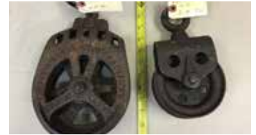
Lot#5617. Hay Trolley Pulleys, F/E/ Myers #H-411 and R.M Co.pulley
