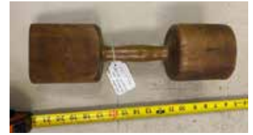
Lot#5843. Wooden Hand Tamper for tamping sand into molds
