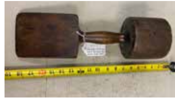
Lot#5842. Wooden Hand Tamper for tamping sand into molds
