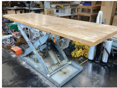
147 American Lifts T36-015 Electric Lift Table, 28" x 83" Top, 1500 Lbs. Capacity
