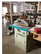
124 Extrema ET-120-3 Shaper, 1 1/8" Spindle, Hydraulic Powered with Forest City Air Powered Feeder
