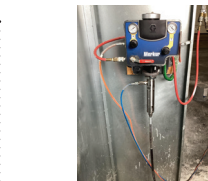
341 Graco Finish Pump with Graco G15 Spray Gun
