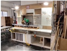
146 Workstation with Lights and Flip Stop Fence
