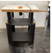
156 Router Table with Bosch PR10E Palm Router, 120 Volt
