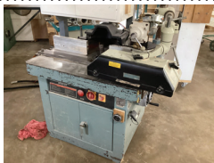
128 Delta 43-791 Shaper, 1 1/8" Spindle, Hydraulic Powered, Extreme 4 Roll Air Powered Feeder
