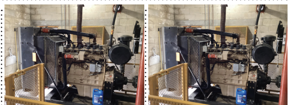
162 Cummins GTA 8.3 Natural Gas Engine with Turbo, WPT Clutch, 175 Hp. At 1800 RPM, 12,540 Hours More Photos →
