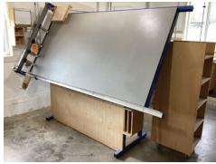
138 Kreg 4' x 8' Face Assembly Frame Table with Air Clamps
