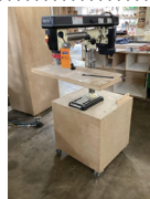
133 Shop Fox W1669/ W1670 Bench Top Radial Drill Press, 115/230 Volt, with Caster Base Stand
