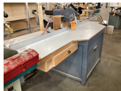
125 MVM DM-10 Crosscut Saw, Air Powered, Extension Table with Flip Stop Fence
