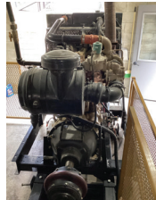
162 Cummins GTA 8.3 Natural Gas Engine with Turbo, WPT Clutch, 175 Hp. At 1800 RPM, 12,540 Hours
