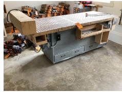
139 34" x 84" Down Draft Sanding Table with Sanding Lights, Electric Powered
