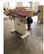
136 Ritter R911 Edge Sander, 6"x109" Sanding Belt, Hydraulic Powered
