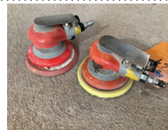
64 2 - 3M 12,000 RPM Random Orbital Sander, 3/16 Orbit
