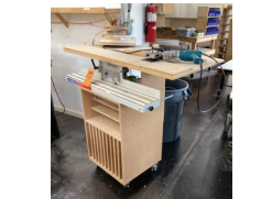
155 Virutex Edge Bander Maksiwa RBB.1000 Edge Trimmer with Cabinet Base, Electric Powered
