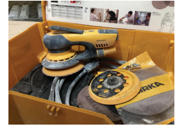
294 Mirka Direct Electric Random Orbital Sander, 3/16 Orbit Central Vacuum
