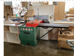
131 General 18" Upcut Saw with Extension Table And Flip Stop Fence, Hydraulic Powered
