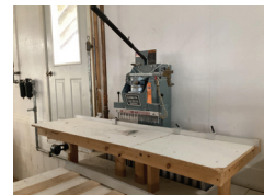
126 Delta 32-325-13 Spindle Line Boring Machine, Air Powered, With Table and Flip Stop Fence
