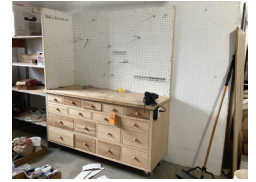
288 25" X 74" Work Bench With Vise, Dovetail Drawers Extension Slides
