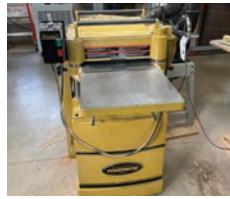
3 Powermatic 15HH 15" Spiral head planer 230V-1phase serial# 1509015HH5918
