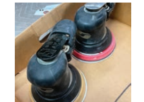
58 2-Dyna brade Air sanders 12,000 RPM 3/32 and 3/16 orb
