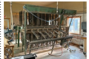
26 Taylor Clamp Carrier 40 section 32" clamps air operated serial# X780
