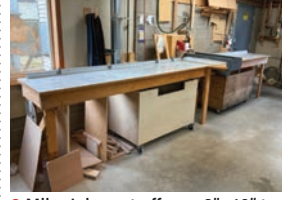
9 Mike Jeka cut off saw 2"x16" top with neat stop fence and stops air power
