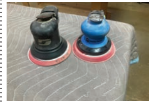
56 2-1-Dyna brade / 1 master power Air Sanders 12,000RPM 3/32 orb
