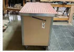
14 Sand Pro model# M4826 26"x 48" down draft table 110V-1phase serial# 7433-7145
