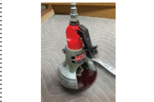
61 MVM Air router Sioux brand 1/4" collet 25,000 RPM
