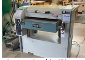
8 Stonewood model # STC 720 MH 30" spiral head planer 220V-3phase serial# 190140, 2 years old
