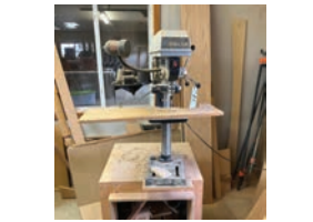
19 Delta model# DP300L 12" Bench top drill press 120V-1phase
