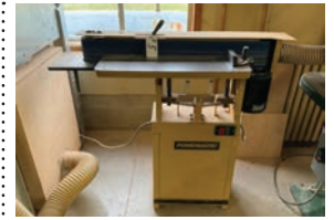
5 Powermatic #13 6x89 Edge sander 115/230V -1phase Serial#4100132589
