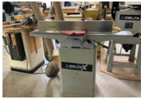
2 Delta Model #37-866x 6" straight knife jointer 120/240V 1 phase, serial# 26252-2008-44 xl
