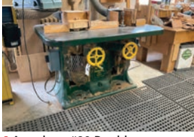
6 American #20 Double Spindle shaper 1 1/8 spindles 230/460V-3phase
