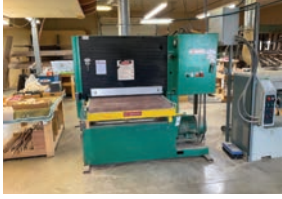
11 TimeSaver 137-1HD 37" Single-head wide belt sander 230/460V-3phase serial# 20405Y
