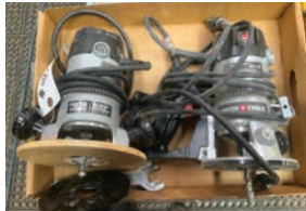
48 2-Porter cable routers 1/2" Collets 120 Volt 1phase
