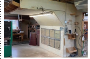
15 Built in Sanding booth includes fan and filters 8' wide x 9' high
