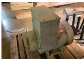
124 Lima Mac Generator 40rw/ 120/240/ Amps 120serial# LM358268-0101
