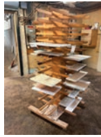
145 Finish room drying rack carts
