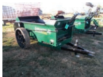
LOT 1507 New Manure Spreader Lancaster Manure Spreader, 25 bushel, 2 wheel, steel wheels, ground drive
