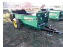
LOT 1505 New Manure Spreader Lancaster Manure Spreader, 50 bushel, 2 wheel, air tires, ground drive
