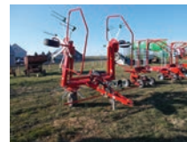
LOT 1511 New Hay Tedder Enorossi Tedder, 19' PTO drive, hydraulic lift, SN 202101321
