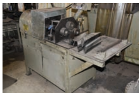
LOT 306 Twister Used to roll brake bands|Form neckyoke rings|Set up for hydraulic
