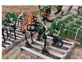
LOT 1184-1187 Cultivator Shank Kit Basic Corn Shank Kit for Cultivator, with finger weeders & all shanks needed for corn
